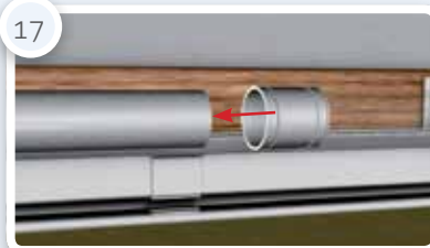
Setting of pipe connector, attend to straight and clean cuts of pipe
