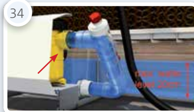
Setting of water connection and pump cover
