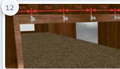
Distance between top brackets max. 75 cm
