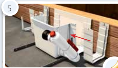
Setting in and glueing of housing for supply unit
