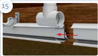
Add pad guide couplers and rear pad guide profiles to needed length
