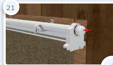
Glueing transition piece and setting sealing cap on end of piping
